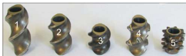
Figure 2. Elements of extruder screw configuration.
